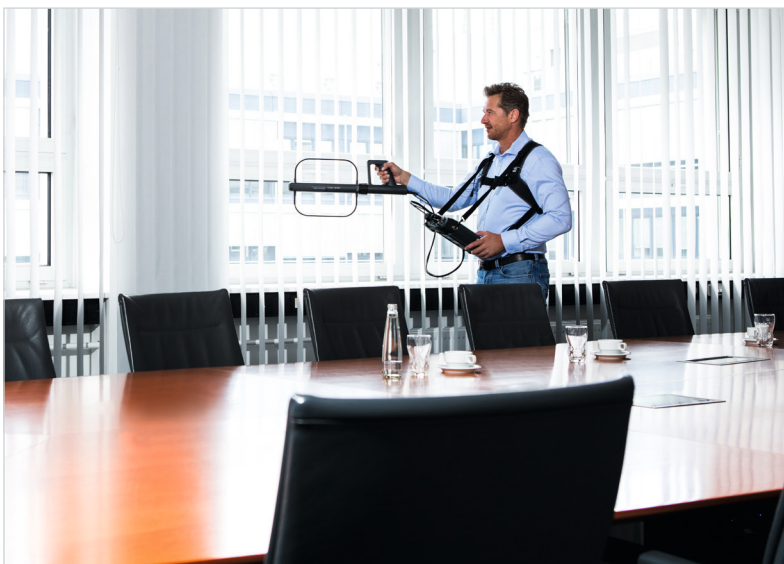
Finding bugs with the R&S®PR100 and the R&S®HE400 handheld directional antenna.
