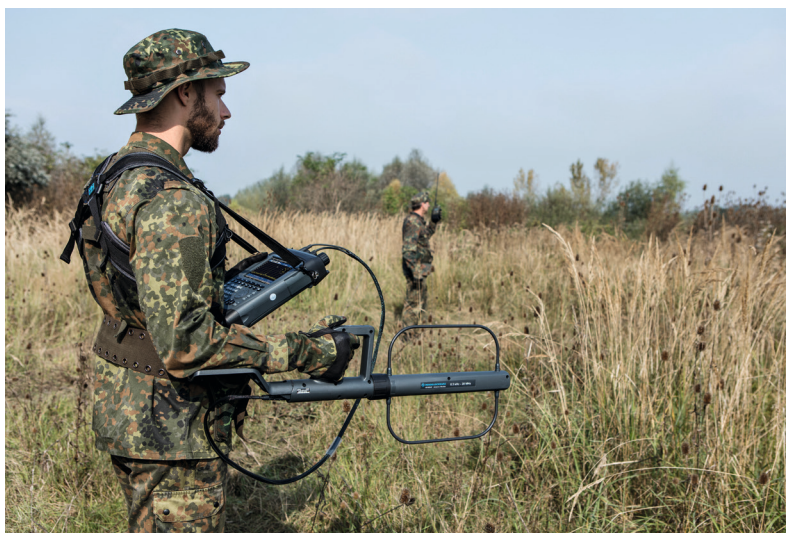
Tracking telltale signals with the R&S®PR100 and the R&S®HE400 active directional antenna.
